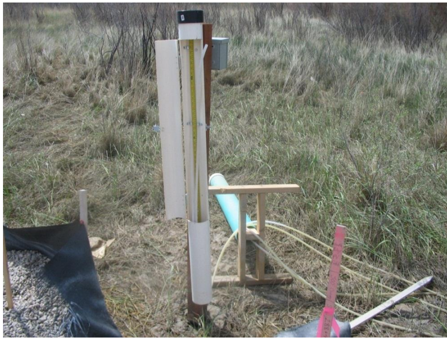
Figure 3-6. Manometer Gauge Box
